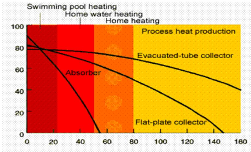
Figure: Graph of efficiency ( $\eta$ ) and Temperature (T) ranges of various type of collector (Solar Radiation: 1000 W/m<sup>2</sup> )
